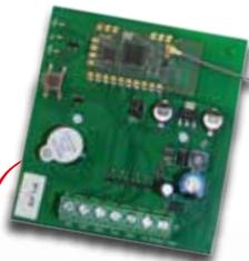
**RICEVITORE LINK-R4 (decoder 4 CH)**
