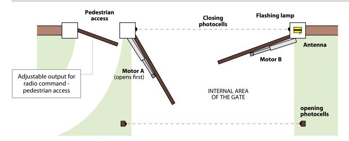
The system must have a physical limit in the opening and closing movement
