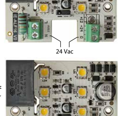
**COLLEGAMENTO PER 12Vdc, 24Vdc e 230Vac****CONNECTION TO 12Vdc, 24Vdc and 230Vac****POUR LE RACCORDEMENT AU 12Vdc, 24Vdc, 230Vac****VERBINDUNG FÜR 12Vdc, 24Vdc, 230Vac****PARA CONECTARSE A 12Vdc, 24Vdc, 230Vac**
