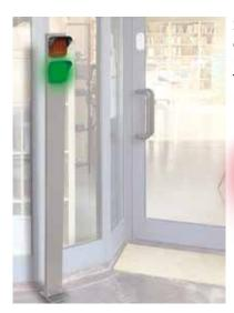
Suitable for small/medium user environments and ussi. Red/green traffic light signaling is controlled by an 868 Mhz two-channel radio transmitter. The operator manually counts the number of users in the area and selects via the transmitter the access or stop colors. The special conguration of the radio receiver eliminates the possibility of simultaneous lighting of the lanterns, and each channel of the transmitter controls the single colours.
