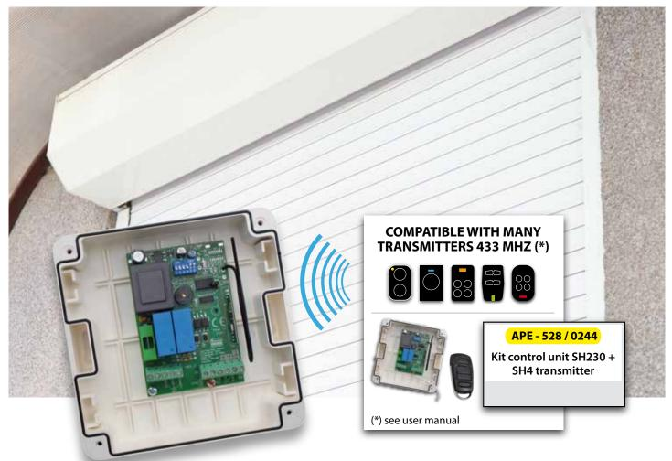
SH230 is an electronic control unit with an **integrated receiver** compatible with all the 433 Mhz fixed codes and some 433 Mhz rolling codes (\*). It is easy to install and to program: it has **TWO inputs for command devices** and 2 safety inputs (1 with normally closed contact and one for safety edges 8,3 k $\Omega$ ).
