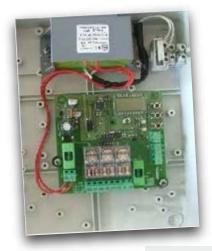
The **TRAFFIC CONTROL** control unit enables the management of traffic light systems two-way, thus with up to two traffic lights with 2 or 3 lights (230V or 24V).
