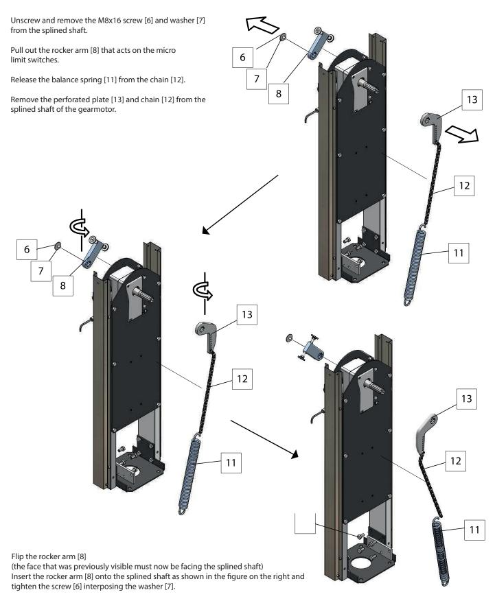
Flip over the perforated plate [13] with the chain attached (the face that was previously visible should now face the splined shaft).
