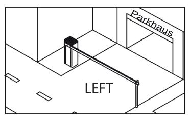
We indicate as 'RIGHT' a barrier that, when looking at the automation from outside the driveway, is installed to the right of the driveway.
