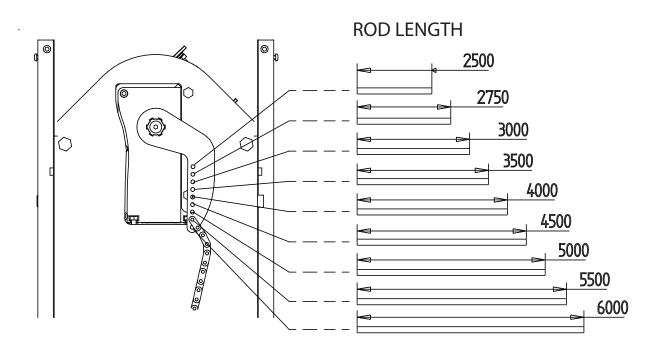
Verify that the chain is connected to the lever in the correct position according to the length of the rod that is to be installed on the barrier.
