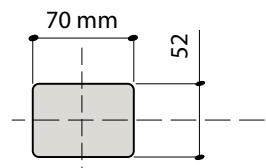
The PFZ is a fixing base without overall dimensions. Necessary if you want to install the column touching the wall. Accessory to replace the 115x85 mm base as standard on DORICA 50, DORICA 50 CAP and DORICA 100
